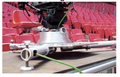
camera and seat, on the same axis and pans over 360° at a very low level, providing easy operation and reducing disturbances due to its central cable feeding.
